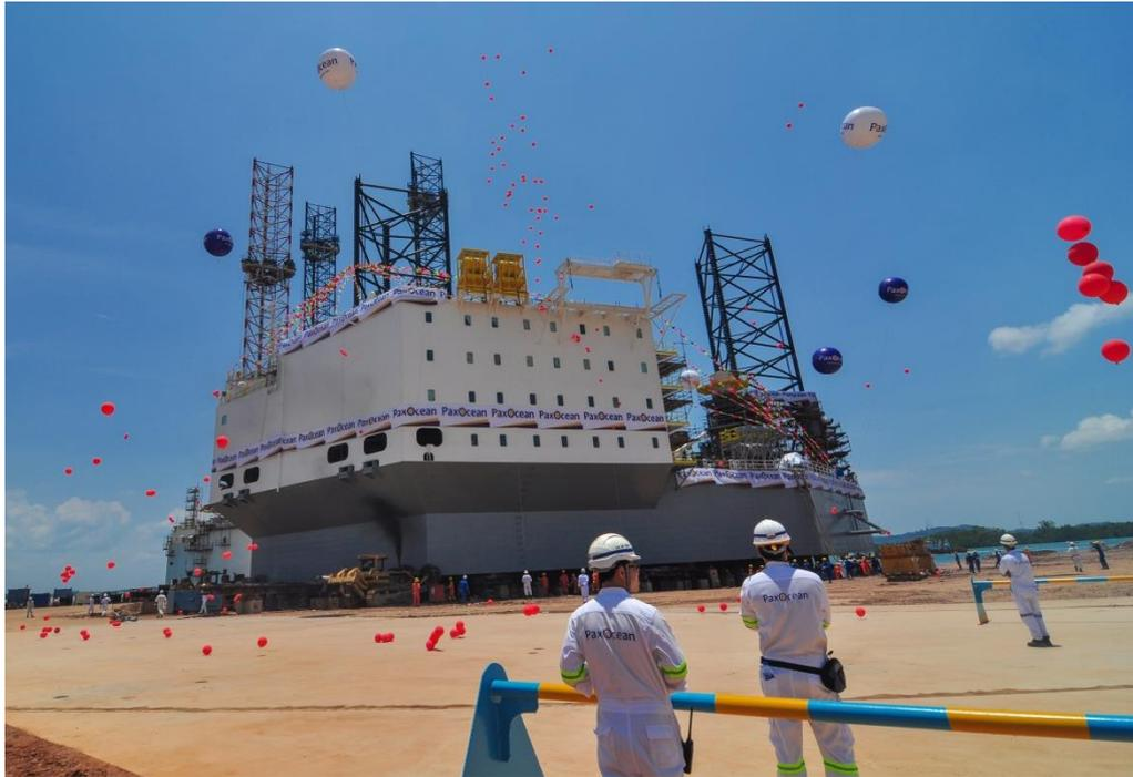
Scheduled for delivery in the second half of 2015, ABS-classed GustoMSC CJ46-100XD Jack Up Rig is capable of drilling at a water depth of 375 feet with an accommodation capacity of 120 personnel. The rig is also equipped with NOV drilling equipment and powered by five units of generators producing 7.5 MW of electricity. The three API2C certified offshore cranes of 50 SWL provide ample heavy lifting capacity for the rig's future offshore operations.
